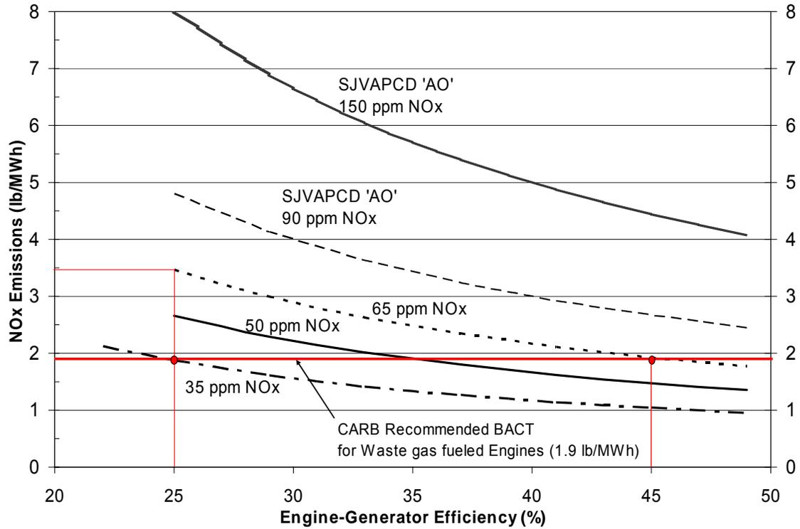
Figure 3. NOx emission rate vs. efficiency for given exhaust concentration (concentrations are at 15% O<sub>2</sub>)
